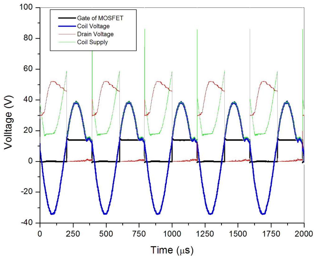
Fig.7. Waveform at the MOSFET Gate, Drain, Coil-high side and across coil
