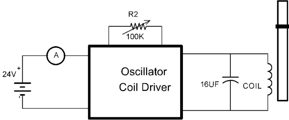
Fig.6. Setup for resonance
