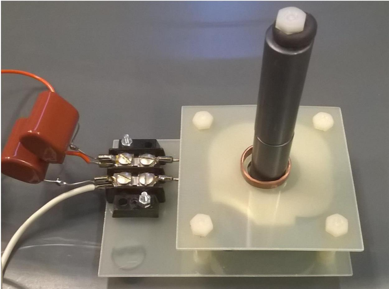
Fig.4. Coil with 16 micro Farad capacitor in parallel
