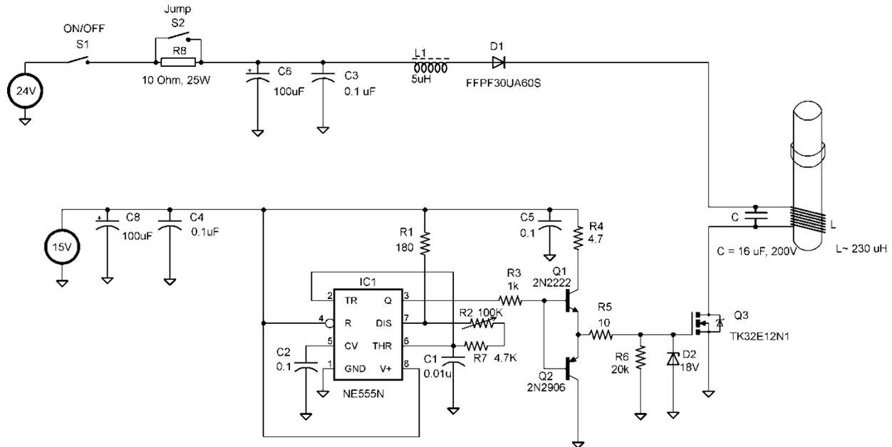
Fig.1. Circuit diagram of the ring launcher
